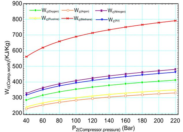
Figure 4: Compressor work input versus compressor pressure for various gasses
