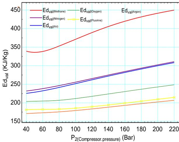
Figure 8: Exergy destruction of J-T valve versus compressor pressure for various gases
