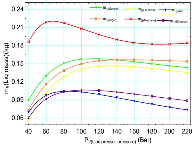
Figure 3: Liquefied mass ( $m_s$ ) versus compressor pressure for different gasses
