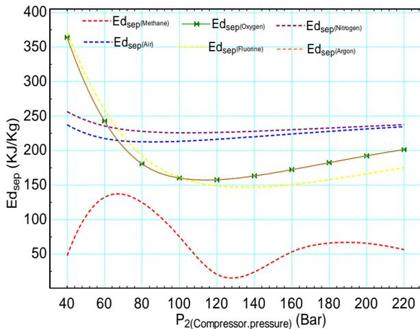
Figure 9: Exergy destruction of separator versus compressor pressure for various gases
