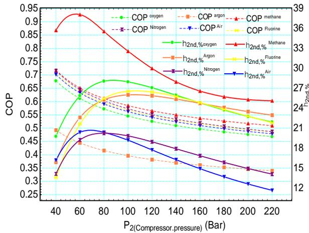
Figure 2: COP and the exergy efficiency versus compressor pressure for various gasses
