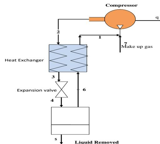
Figure 1: Schematic diagram of Linde-Hampson cycle
