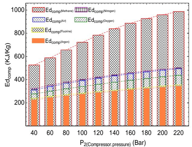
Figure 6: Exergy destruction in compressor versus compressor pressure ratio
