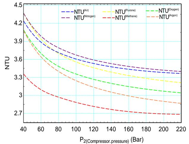
Figure 5: NTU versus compressor pressure for various gasses
