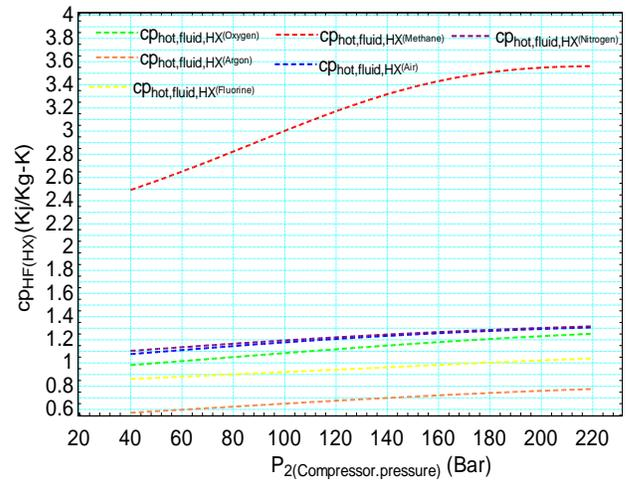
Figure 10: Specific heat of hot fluid versus compressor pressure for different gases
