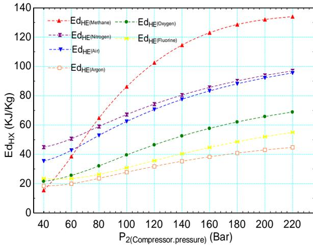
Figure 7: Exergy destruction of HX versus compressor pressure for various gases
